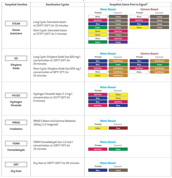
Tempilink® is most commonly used in producing Type 1 and Type 2 (e.g. Bowie-Dick test packs) indicators. The inks are also used in creating Type 3, Type 4, and Type 5 indicators.
